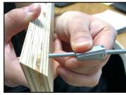
Screw the Wings(D) onto the Bolts(C) as shown. Screw the wing about 1/3 of the way up the bolt.
